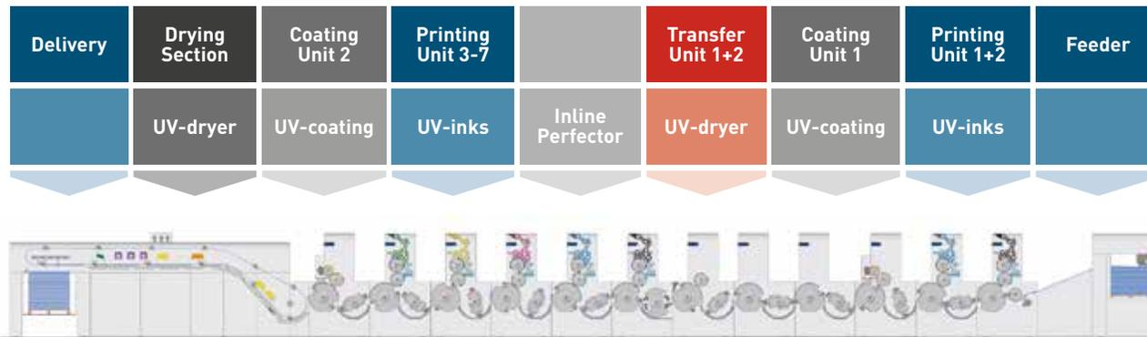
In straight mode this configuration can apply opaque white or primer with the coating module before perfecting.
