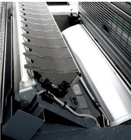
Fig. 2: Blast air blows the sheet flat on the cylinder during inspection.
