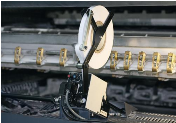
Fig. 3: Marking of defective sheets with strip inserter in the delivery.
