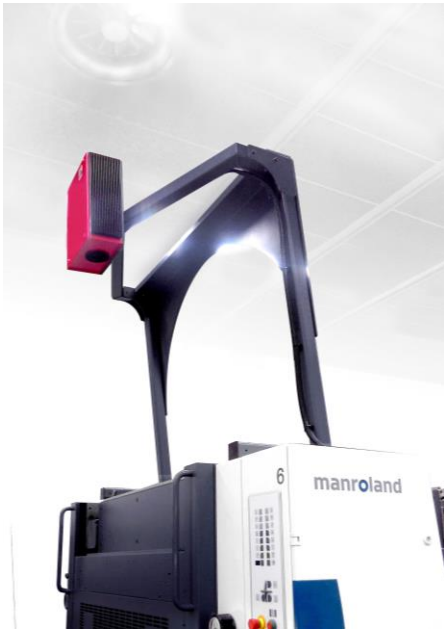
Fig.1: High resolution camera above the last printing unit.
