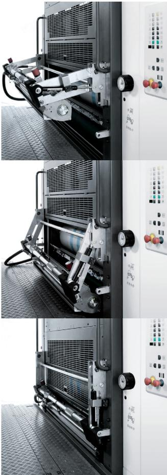
Within 5 minutes, the ROLAND InlineCoater smart makes a coating unit out of a printing unit.
