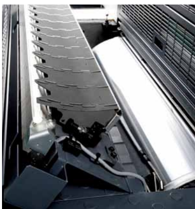
Blast air holds the sheet flat on the cylinder during inspection.
