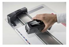
The measuring device is detachable for handheld functions.
