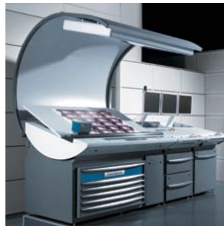
ColorPilot – colour measuring and control systems with combined densitometrical and colorimetrical measuring technology.
